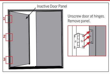
a. Remove the inactive door panel by unscrewing the door from the hinges.
