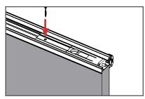
d. Secure the strike support with the included screw. It should fit against the flush bolt in the unlocked position. 2 of 3
