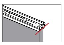
c. Slide the new bolt into the astragal body. The end of the bolt should be flush with the end of the astragal.
