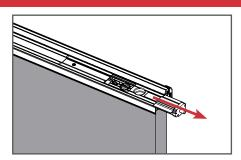
Slide the bolt to replace out of the astragal using the finger notch on the bolt. (Lower bolt shown in image).
