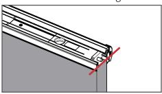
b. When the bolt is retracted (unlocked), the end of the bolt should be flush with the end of the astragal.
