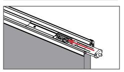
a. Slide the new bolt into the astragal body, ensuring the inner end of the bolt slides under the locking bracket.
