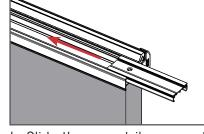
b. Slide the new strike support bracket into the astragal body.
