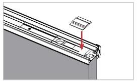
\*Note: If replacing the lower bolt, install a new corner pad (purchased separately) at this step.
