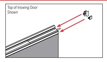
b. Install the trim cap and spacer to the top.
