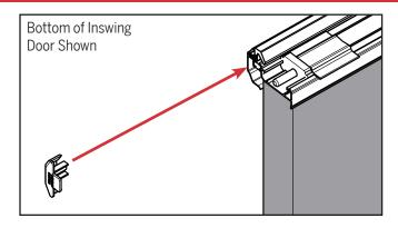
a. Install the new trim cap to the bottom of the astragal. For outswing doors, install the new spacer to the bottom as well.
