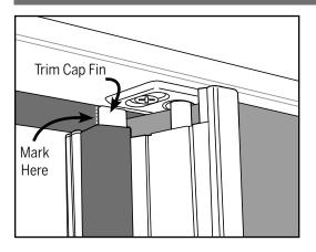
**a.** Close the inactive door. Mark the location where the trim cap fin meets the header weatherstrip.
