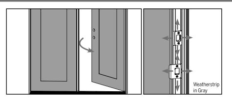
**b.** Close both the active and inactive doors and engage the deadbolt to ensure the door closes and locks completely. If not, adjust the location of the strike/ deadbolt plate.
