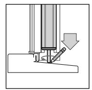
Close inactive door until weatherstrip on header is compressed. Push upper and lower bolts so the pins come in contact with the header and sill. Mark contact points.
