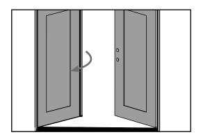
**a.** Close the inactive door and engage the upper and lower bolts. Ensure the bolt pin slides into the head and sill bolt receivers without obstruction. If not, adjust the location of the bolt receivers.
