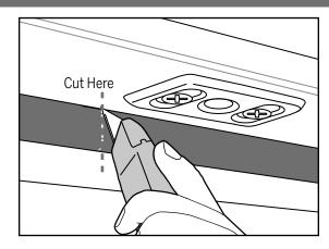
**b.** Open the inactive door and use a utility knife to cut the header weatherstrip on the mark made.
