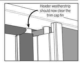
**c.** Ensure that the trim cap fin makes contact with the active door panel when the door is closed, maintaining the integrity of the seal.
