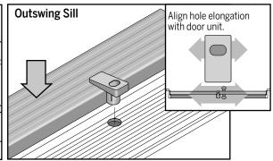
Hole Diameter: 3/8" Hole Depth: At least 1-3/8" Hole Diameter: 5/8" Hole Depth: 3/4"
