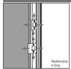
**a.** Close both doors and determine the exact location of the strike and deadbolt plates. Loosen the securing screws and adjust the placement of the plates.
