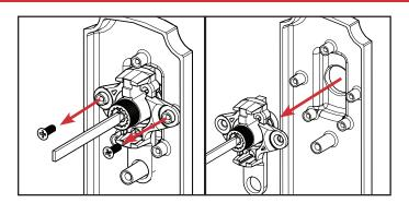
Remove the screws securing the mount into the escutcheon plate and set them aside. Remove the mount and lock cylinder from the handset.
