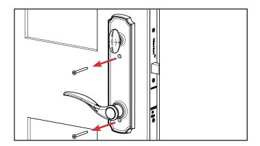
Remove the screws from the interior escutcheon. securing the handset to the door panel. Be sure to hold the exterior escutcheon so it does not fall.
