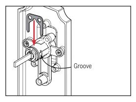
c. Insert the retaining clip into the groove on the cylinder as shown above.
