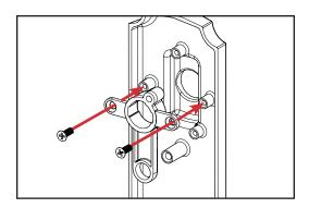
a. Align the new mount into the escutcheon as shown above. Use the screws removed from the previous mount to secure the new mount into the escutcheon.
