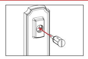
b. Remove the key from the new lock cylinder. Insert the lock cylinder into the mount from the exterior of the escutcheon plate with the smooth side towards the bottom of the mount and the raised portions on the top and side.
