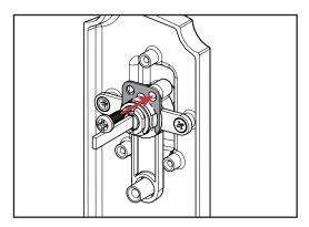
d. Secure the lock cylinder and retaining clip with the  $\#8 \times 3/8$ " self-tapping screw.
