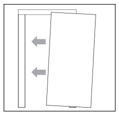
a. Realign the door panel with the hinges in the frame.
