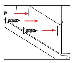
c. Close the door panel and check that the door bottom meets the sill cap to provide proper weathersealing. Once the positioning is set, secure the door bottom to the door with the screws provided. Position screws in the center of the slots.
