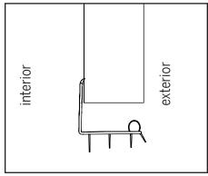
a. Orient the door bottom with the door panel as shown above.
