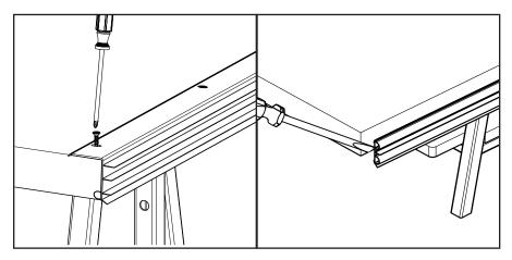
a. Remove the old door bottom from the door panel by removing the screws, if it was a screw-on door bottom. If the door bottom was staple-on, you may need to pry it off with a flathead screwdriver.
