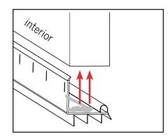
b. Using hand pressure, press the door bottom flush against the bottom of the door panel. Make sure the door bottom is flush down the length of the panel square at the ends.
