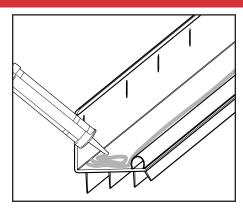
b. Apply exterior grade caulking along the edge of the door bottom that will be facing the exterior of the home. Thoroughly caulk each end of the door bottom.
