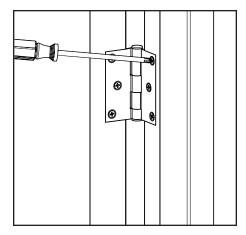
b. Reattach the hinges to the jamb with the screws. Confirm the door operates properly.
