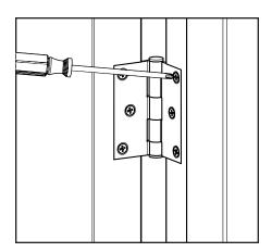
a. Open the door and locate the hinges. Using a Phillips screwdriver or drill, remove the screws from the hinge plate on the jamb.
