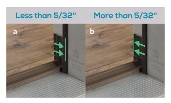
**a.** If your strike margin measurement from Step 1 is **less** than 5/32", align the corner pad with the weatherstrip kerf.
