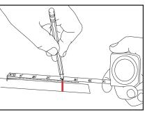
b. Measure the length of the trim strip to be replaced, or the length of space where the trim is missing.
