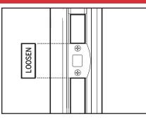
b. If the trim adjoins the strike and/ or deadbolt plate, loosen the plates to allow the trim to fit under the edge of the plate. Once the trim is inserted, tighten the screws.
