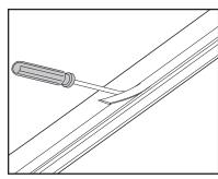
a. If replacing existing trim strip: Remove trim stip by prying up one end with a flathead screwdriver and peeling away from the astragal body.
