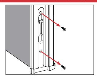
Remove the mounting screws securing the existing flush bolt and then remove the existing flush bolt.
