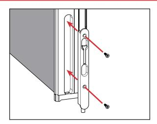
Insert the new flush bolt into the pocket, flush against the astragal. Secure in place with the mounting screws.
