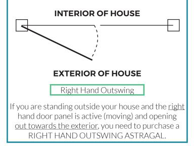
Astragals should be ordered based on the handing and swing of the <u>active</u> (moving) door panel.
